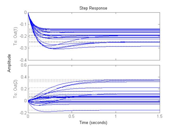
The command stepplot can be called directly on a uss object. The default behavior samples the uss object at 20 instances, and plots the step responses of these 20 models, as well as the nominal value.
